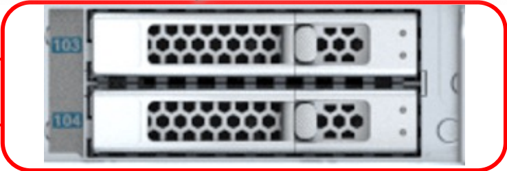
PCle Storage Riser Close-up - Rear View
